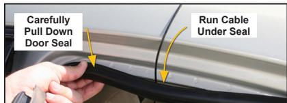
For a more professional-looking installation, run the antenna cable under the door seal. Carefully pull down the door seal. Run the cable under the seal and push the seal back into place. This prevents constant wear and tear on the cable as the door opens and closes. The antenna cable is small enough to easily tuck under the door seal or plastic molding.
