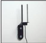
Attach the suction cup bracket to the inside of a window so that the cable will reach the location of the Sleek. Place the bracket as high on the window as possible for best performance.
