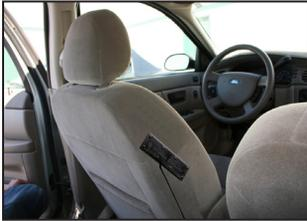
Place the Low-Profile Antenna on the side of the driver's seat for maximum performance.
