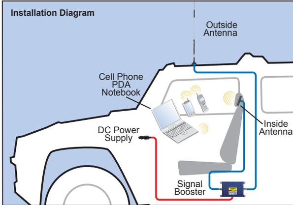
**Warning:** In a wireless installation, do not plug the Signal Booster directly into the cell phone and/or data card using an antenna adapter. It will damage the Signal Booster, cell phone and/or data card.
