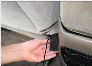
**Warning:** The inside antenna must be installed with a separation of at least eight inches from all persons and must not be located in conjunction with any other antenna or Signal Booster.
