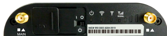
SIM SLOT/ON-OFF / LEDs / SIGNAL STRENGTH COR IBR600
